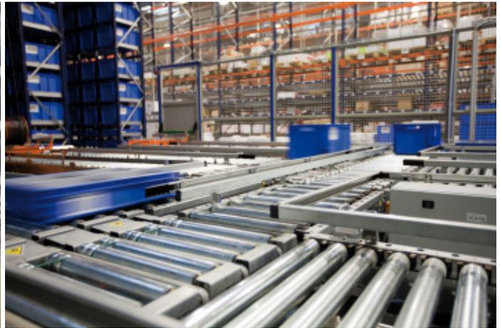
All processes related to picking begin in this area and are guided by the Mecalux Easy WMS warehouse management system. The first step is placing the boxes in the order prep positions located at the back and that also form part of the conveyor.
