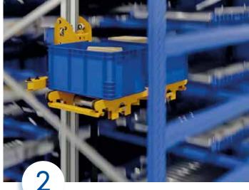
Once the tote is in the cradle, the shuttle moves to the **elevator**, **which lowers the goods** to the outgoing conveyor on the bottom level.
