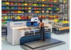
This solution enables operators to prepare large volumes of orders simultaneously and ergonomically. Totes arrive at the station's upper level, where the operator retrieves the required SKUs and places them in the boxes on the lower level to complete orders. This process helps minimise errors.
