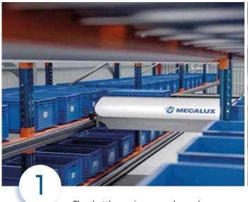
The shuttle receives an order and travels to the assigned position to retrieve a tote from the racking using its telescopic arms.
