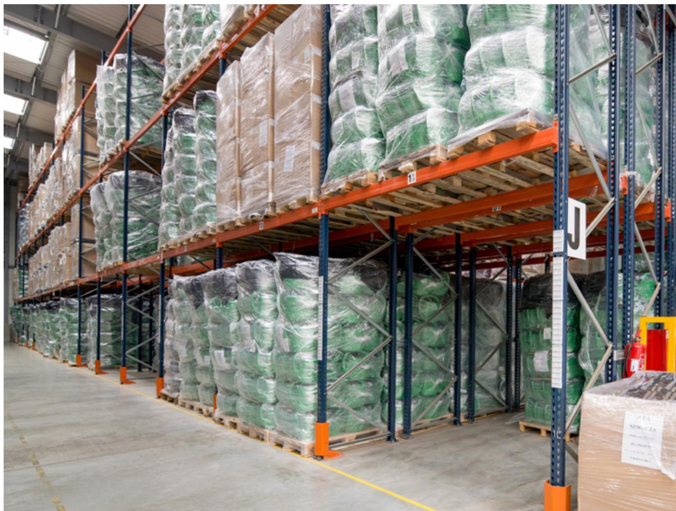
Racking can hold two pallets on either side of the aisle, guaranteeing greater storage capacity
