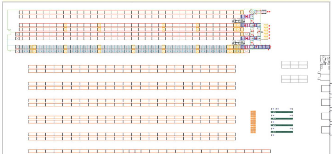
Incoming and outgoing processes in the warehouse are performed using a conveyer circuit that incorporates a pallet checkpoint. This checkpoint is used to check that the dimensions, weight and condition of the pallet meet the specifications of the installation.
