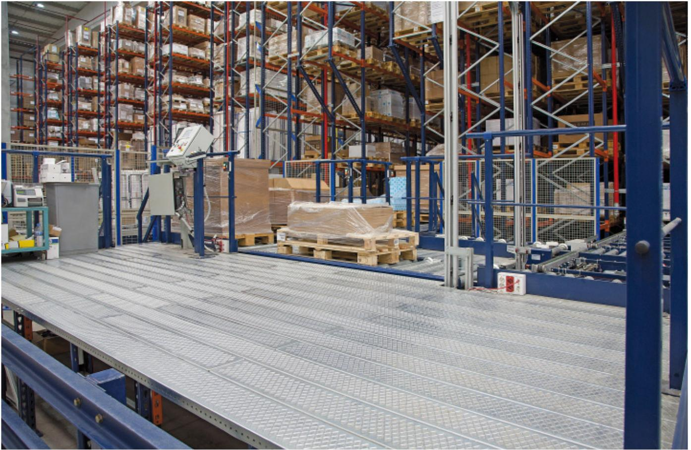
In addition to the picking station installed at the front, 44 live pallet channels have been enabled on the ground level
