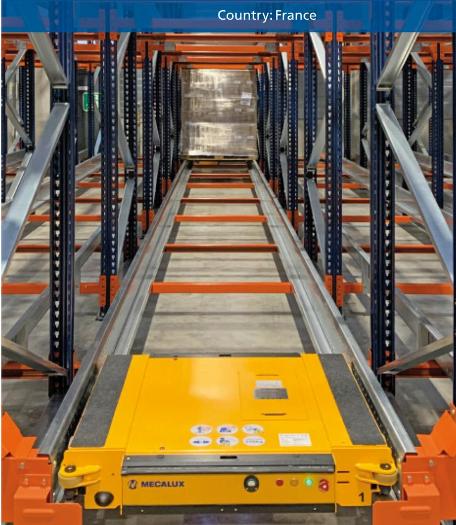
**Sauce manufacturer Manna Foods has renovated its warehouse in Wijnegem, Belgium, with the installation of the Pallet Shuttle system from Mecalux. This solution makes the most of the available space to provide greater storage capacity: 1,120 pallets in just 350 m<sup>2</sup>. The secret? A motorised shuttle tasked with handling the goods, thereby streamlining pallet entries and exits.**
