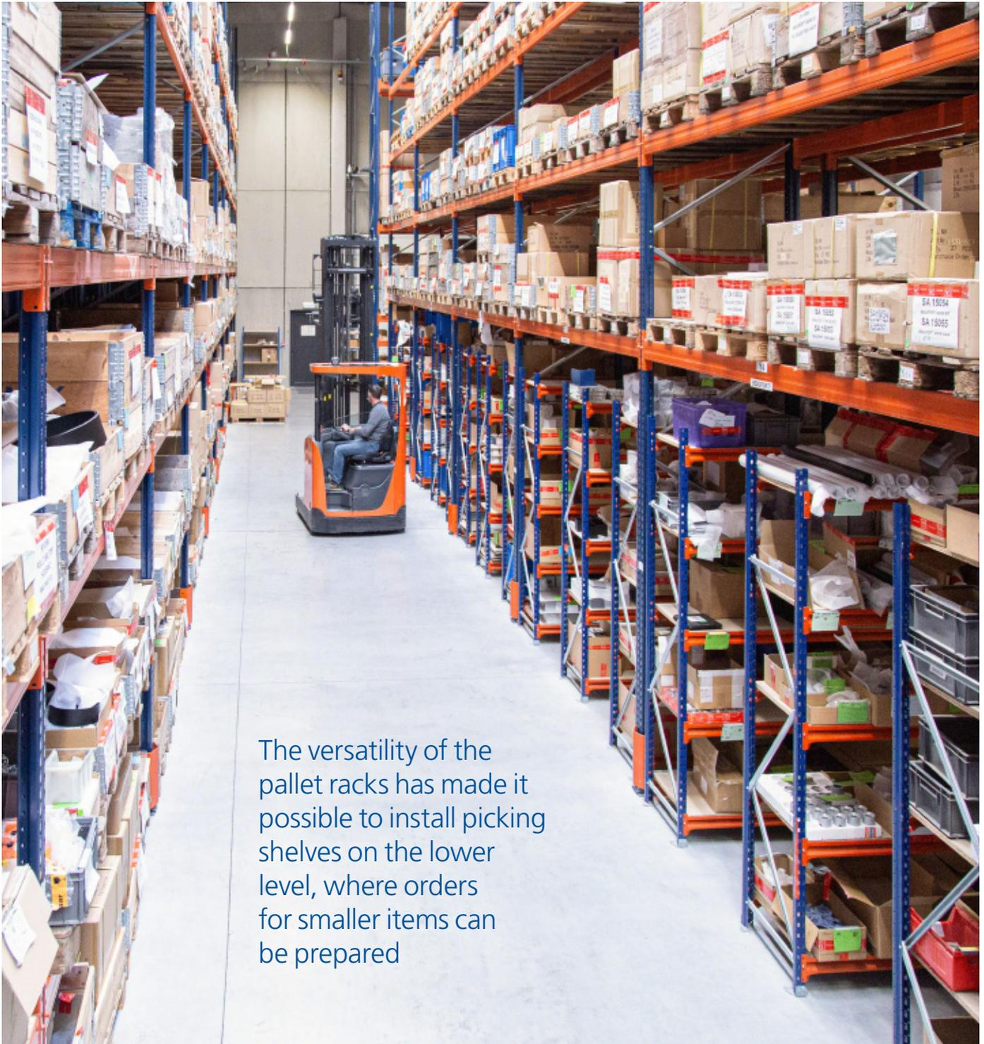
The versatility of the pallet racks has made it possible to install picking shelves on the lower level, where orders for smaller items can be prepared
