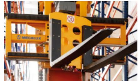
**Extractor element.** The trilateral fork driven by a head moves to the left, right or front to access the load.
