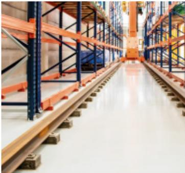
**Guide rails.** Guided by two rails fixed to the floor, it has an eight-wheeled travelling gear that facilitates its movement.
