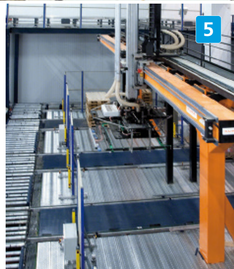
The automated picking robot can prepare high turnover products in small multiples instead of larger groupings. The pallets are fed by the stacker cranes and automated warehouse containers.
