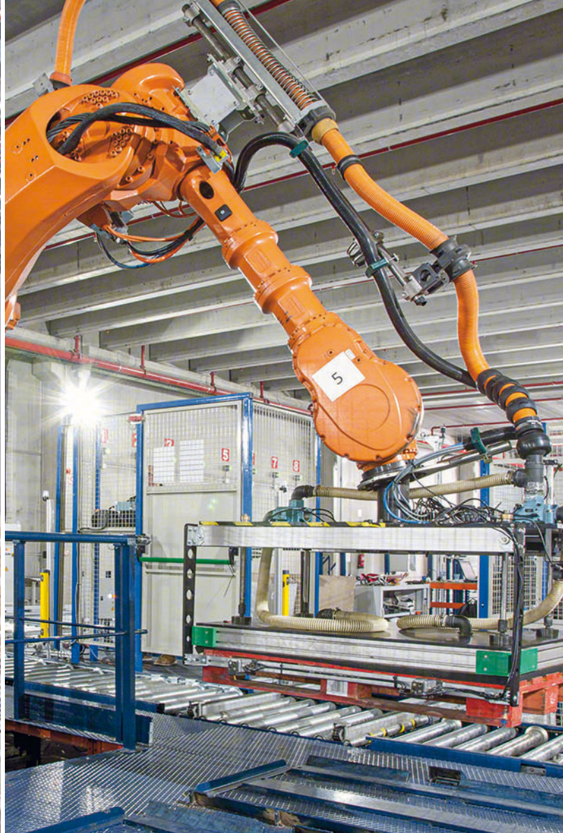
Automatic picking system depalletizer robot operation outline.
