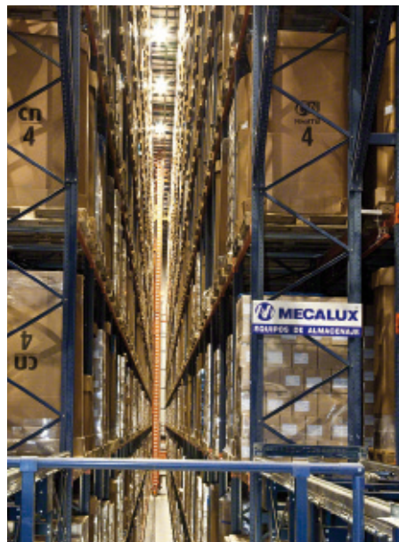
Warehouse with stacker crane.
