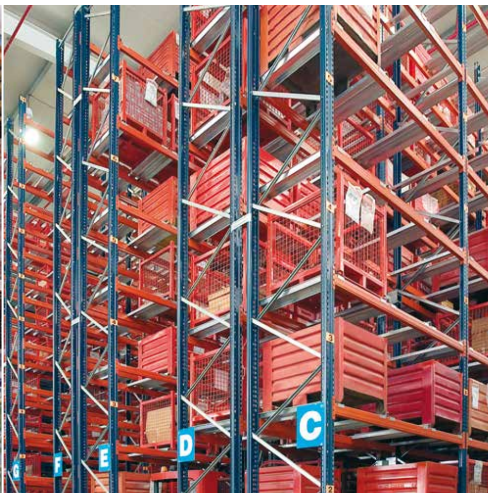
Selective pallet racking system with metal containers
