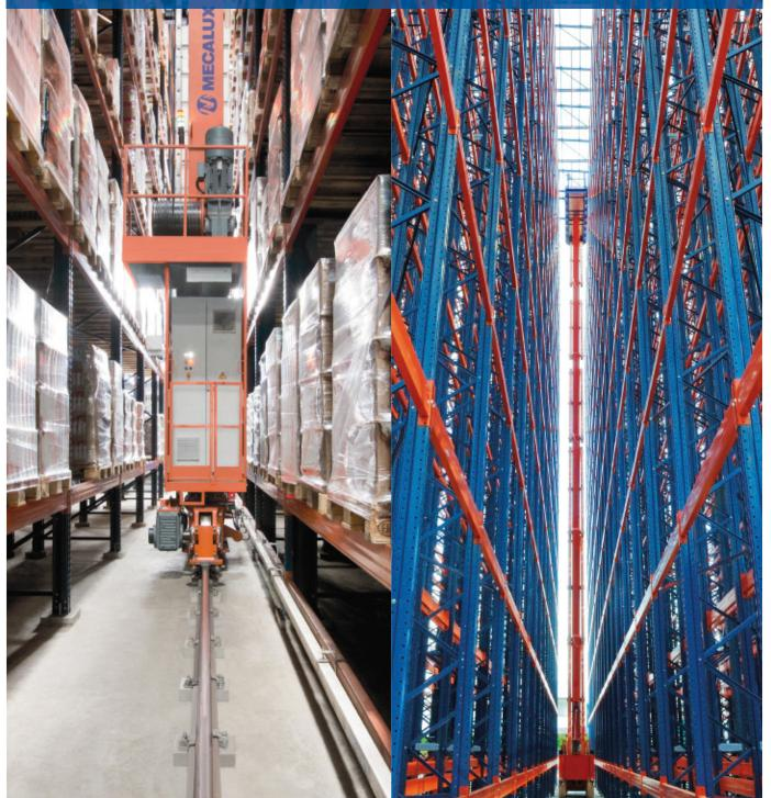
Picture a fully-automated, 32 m high clad-rack warehouse built key-in-hand, with all goods managed smoothly and efficiently by the Easy WMS of Mecalux; then, add storage capacity for 15,428 pallets. That is 'Multisoft' in a nutshell, the 4,400 m<sup>2</sup> sophisticated logistics complex of Lakma Strefa – one of the most cutting-edge chemicals company of Poland–, located in the town of Warszowice, in the Southern region of the country.
